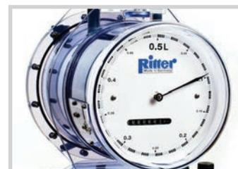
Digital wet gas meter and other sensors can be used for vent gas measurement
